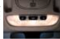
Light panel includes courtesy and two map lights. Standard on all models.
